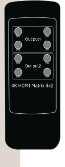
1) The four buttons on Output 1 is the corresponding input source IN1-IN4 which out from Output 1,IN1-IN4 can be switched freely.
